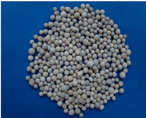
Borosilicate glass nodules developed at CGCRI, Kolkata
